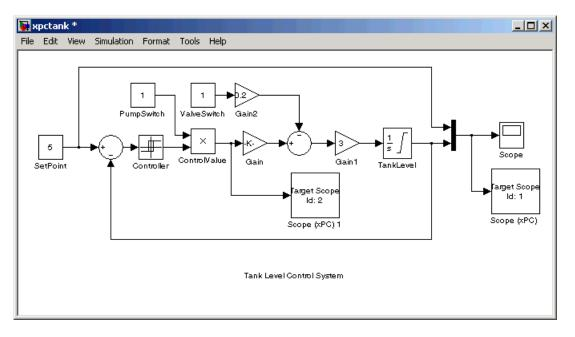
**TankLevel** — The water level in the tank is modeled using a limited integrator named TankLevel.
